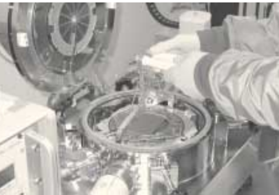
Anodic soldering system – final step when manufacturing MEMS gauges
